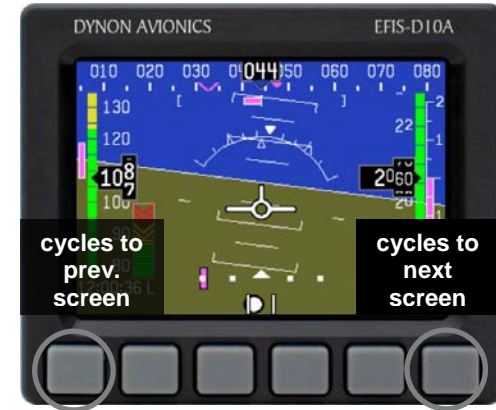
Buttons one and six cycle to the previous and next screens, respectively.
